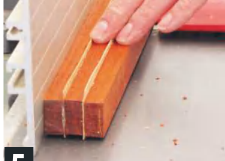
5 Once the glue has dried, plane the face side, then thickness the timber so it finishes at 20mm
